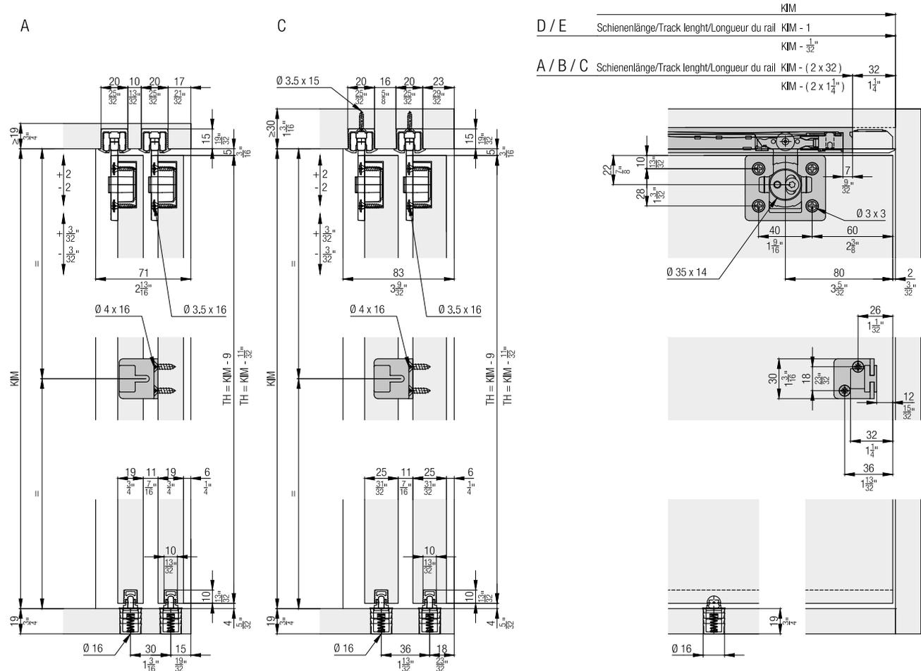
**Set for 2 wooden doors up to 26 kg (57 lbs.), with height adjustment**
