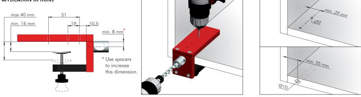
DRILLING SPACERS FOR OTHER PANEL THICKNESSES
