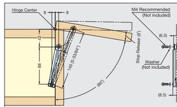
\*Lid stay must be installed parallel to the sidewall.
